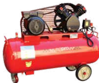
◀ MC30100 - COMPRESSOR AIR 2.25KW BELT DRIVE 100L AGPRO
