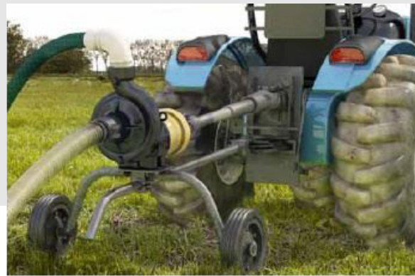
T0-50 Tractor connection with cardan shaft
